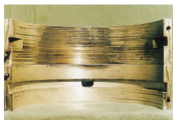
Lagerverschleiß Bearing wear & tear/ Friction bearing Usure de roulements /Palier lisse
